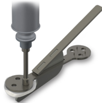
Figure 23: Drilling Peg Holes
